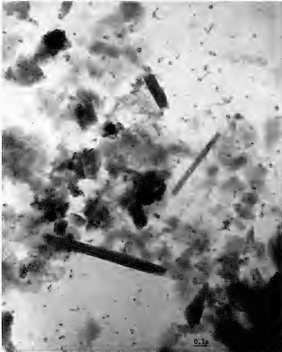
Fig. 5. Electron micrograph of halloysite tubes from the core Capricorn BG 9, 19° 01'S, 177° 46'E. (By courtesy of Shell Development Corporation, Houston, Texas.)
